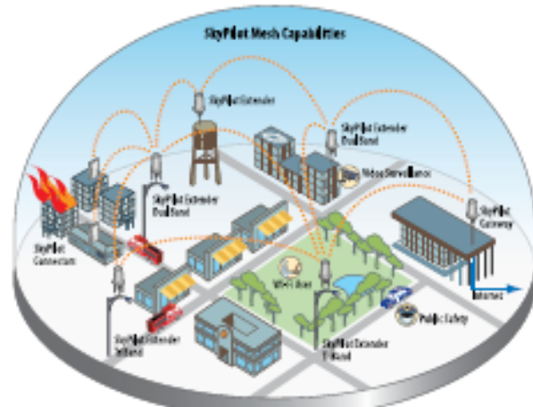
Each SkyPilot Gateway acts as a capacity injector and network takeout point to define a mesh subnetwork as part of the overall SkyPilot network deployment.
