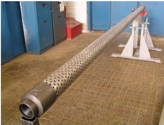
Figura 15. Malla control arena.
