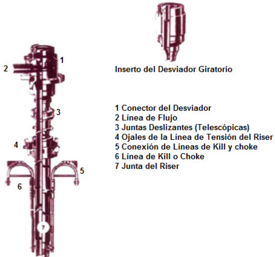
Figura 30 Telescopic slip-joint, choke and kill lines
