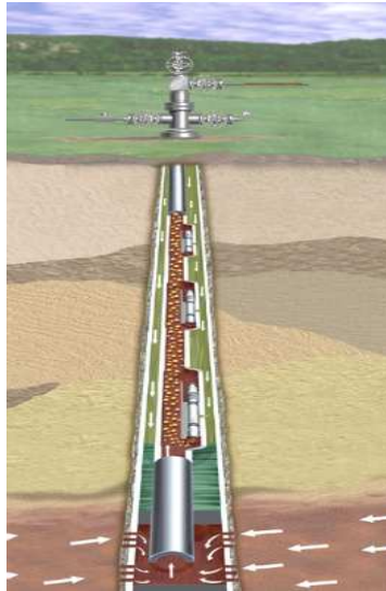
Figura 2. Sistema de gas lift . Fuente: Artificial-lift Systems. Pump up reservoir recovery with the experts in all forms of lift.
