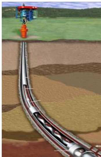
Figura 1. Bombeo por cavidades progresivas. Fuente: Artificial-lift Systems. Pump up reservoir recovery with the experts in all forms of lift.
