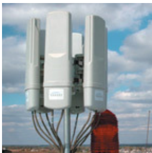
Figura 13. Suscriber Module Advantage 5450SM Canopy.
