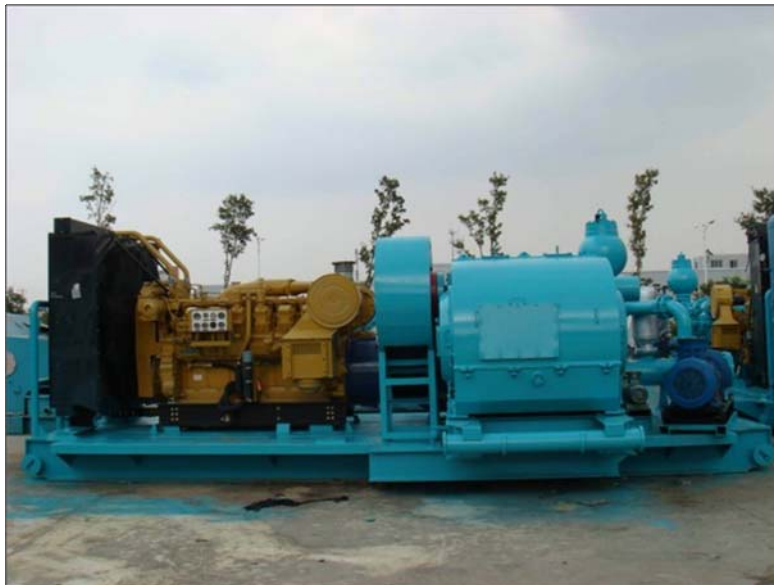
Figura 13 Oilwell 1100 Mud Pump
