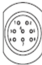
7 Pin Integral or Hanging Connector (male profile) Connection Type: C, M, or J Mating Accessories: • BN 251135 Field Installable Connector • Extension Cable
