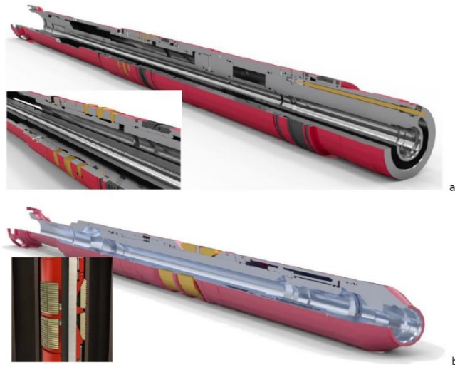
Figura 36. Locking mechanism a. Dual Flow Hanger (DFH), b. Suspension Hanger
