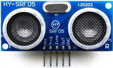
A blue printed circuit board (PCB) ultrasonic sensor module. It features two circular ultrasonic transducers, one labeled 'F1' (transmitter) and one labeled 'R1' (receiver). The PCB is marked with 'HY-SRF05' and '120203'. It has four pins extending from the bottom, labeled 'VCC', 'Trig', 'Echo', and 'GND'. |
