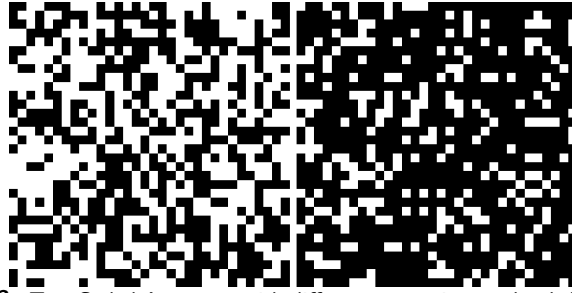
Figure 2.3: Two Coded Apertures with different transmittance level. White pixels allow the light to pass through, while black pixels block the light.
