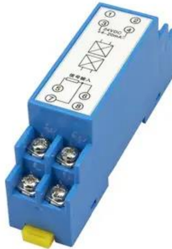
Figura 16. Conversor RTD PT100 a 4~20mA (0°C ~ 150°C) Riel DIN.
