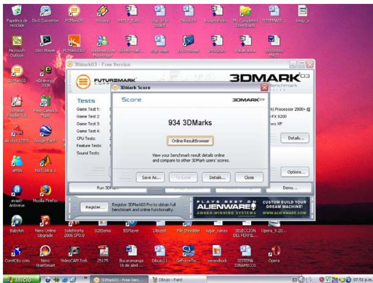
Figura 46. Testeo tarjeta de video GEFORCE FX5200 (128 MB) sin overclocking
