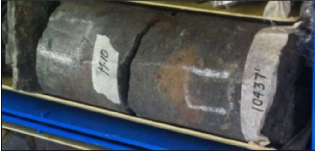
Figura 40. Facies Wackestone, pozo Hormiga-1X, 10437 ft.
