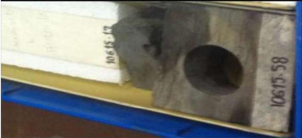
Figura 53. Facies Arenisca glauconítica bioturbada: Hormiga-1X, 10611 ft.
