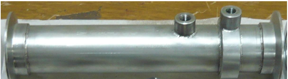
Figura 50. Tubo principal montaje 1 ½ in
