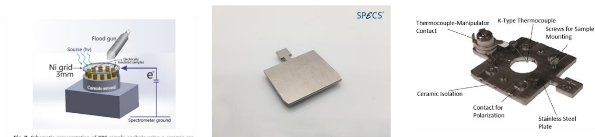
Fig. 7. Schematic representation of XPS sample analysis using a ceramic carousel isolated from the spectrometer.
