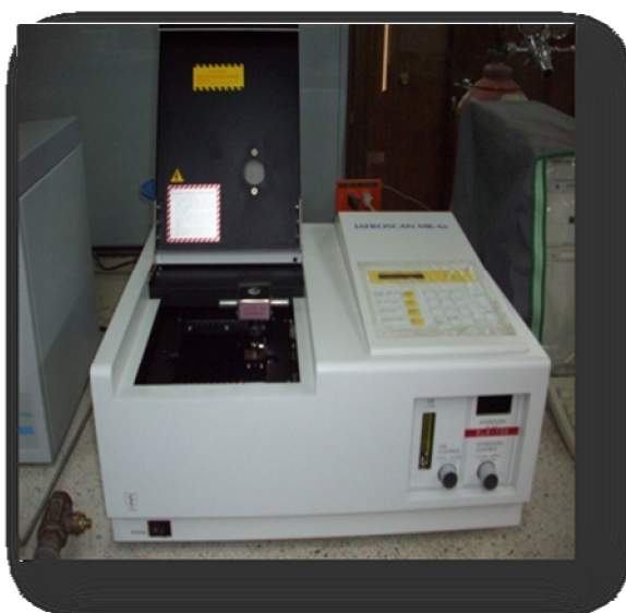
Fotografía 10. Determination of saturated, aromatic and polar compounds in petroleum products by thin layer chromatography and flame ionization detection (IP ST-G-2)
