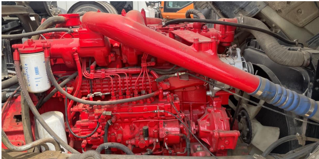
Figura 1 Motor Doosan DE12TIS
