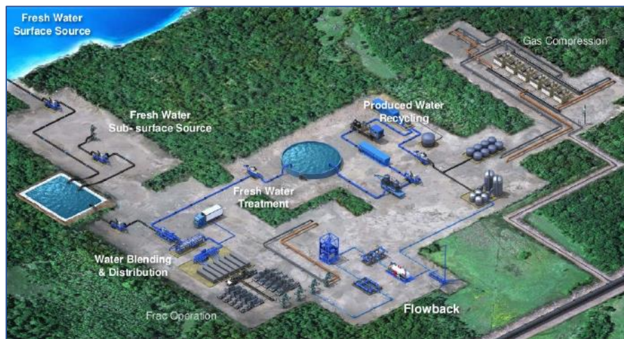
Figura 26. Esquema de fracturamiento hidráulico con tratamiento y reúso de agua de flowback. Fuente: TETRA Technologies, Inc. Technology Advances in the Handling and Movement of Produced Water. Disponible en https://www.tetrathec.com/download/tetra-integrated-water-management-solution-brochure/?wpdmdl=3136&refresh=5dc681d94d5321573290457 .
