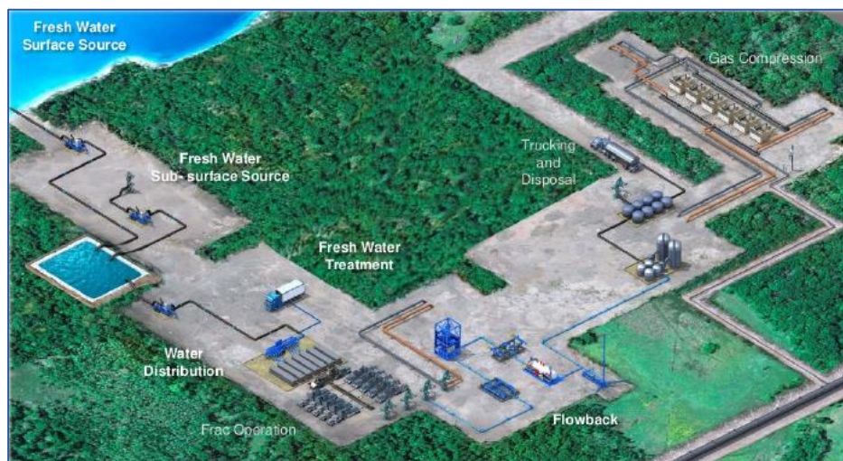
Figura 25. Esquema en superficie del fracturamiento hidráulico sin reúso del agua de flowback. Fuente: TETRA Technologies, Inc. Technology Advances in the Handling and Movement of Produced Water. Disponible en https://www.tetrtec.com/download/tetra-integrated-water-management-solution-brochure/?wpdmdl=3136&refresh=5dc681d94d5321573290457 .
