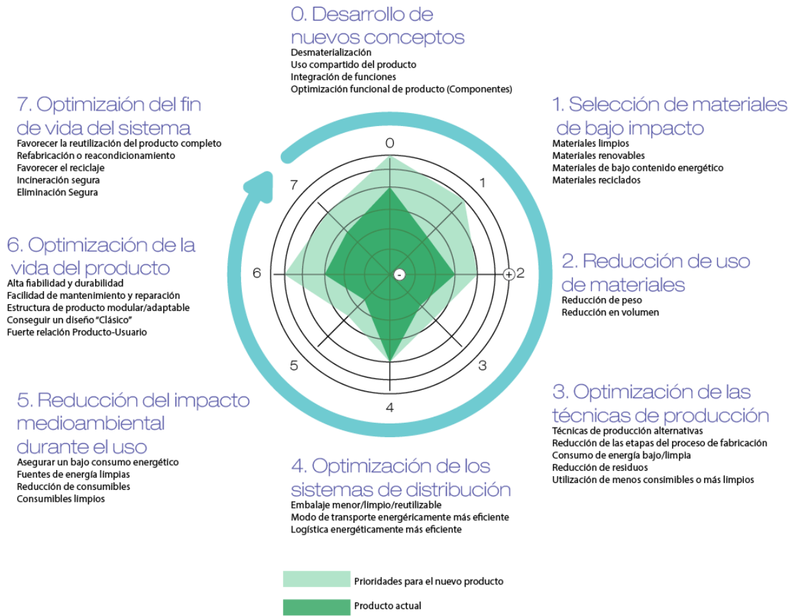
Ilustración 8. Rueda de las estrategias. Adaptada de van Hemel, C., & Brezet, H. (1997). Ecodesign: a promising approach to sustainable production and consumption . UNEP Industry and Environment .
