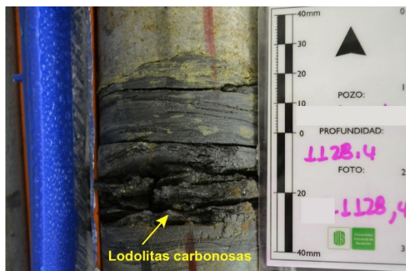
Figura 43. Lodolitas carbonosas a 1128.4 ft.
