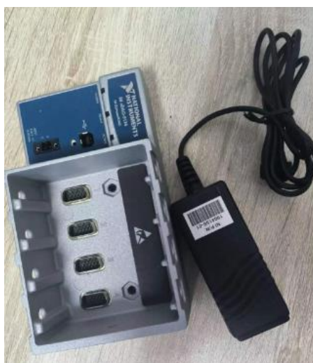
Figura 59. Chasis CompactDAQ 9174 USB 4 ranuras
