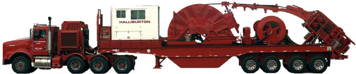
Figura 15. V95HP Quick Rig-up unit.
