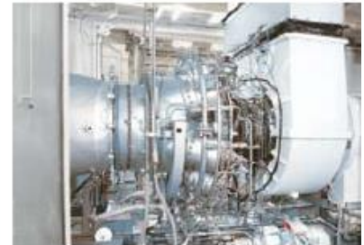
SGT-300 core engine test facility.
