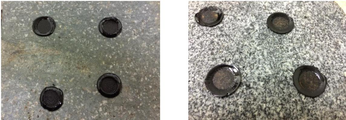
**Figure 12.** Bitumen bond strength specimens after testing under dry conditions for bitumen with aggregate a) AGC and b) AGE.
