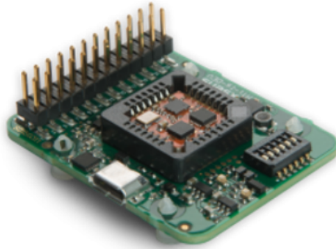
Figura 10: Xsens MTi 1-series Development Board with MTi-3-8A7G6 module.
