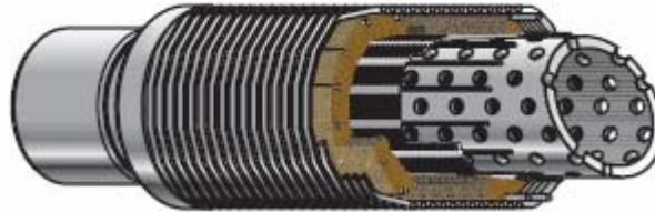
Figura 13.21. Malla Enhanced Low Profile. Tomado de Halliburton Sand Control 2005
