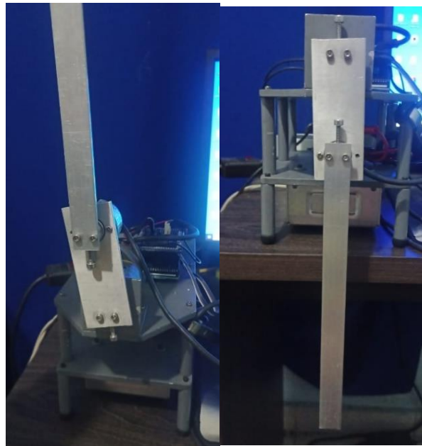
Figure 23. The equilibrium point of Pendubot
