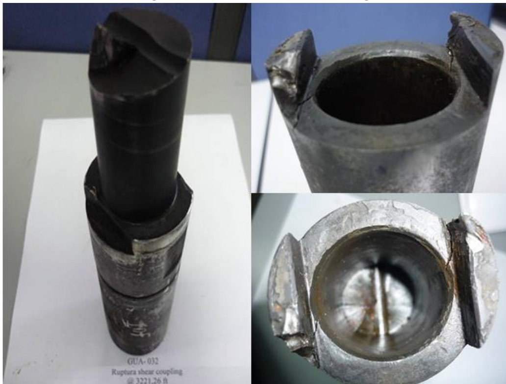
Figura 50. Falla Shear Coupling GUA-032
