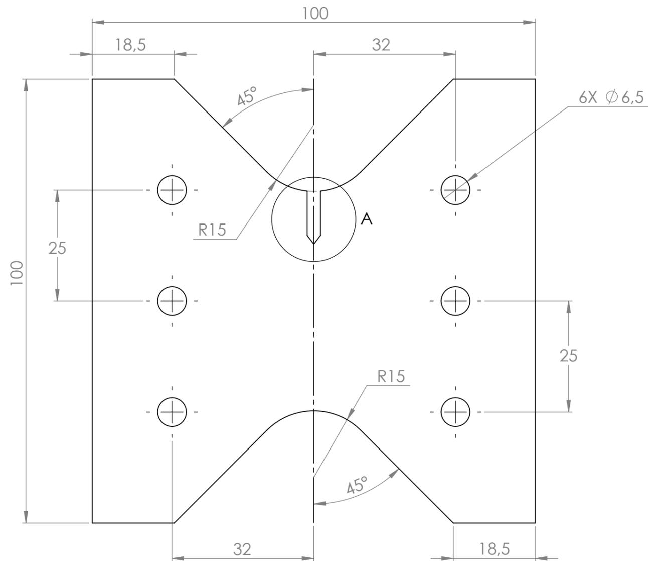
PROBETA ENSAYO ARCAN
