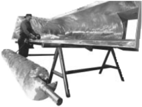
USDA Approved Stainless Steel Screw Conveyor for Handling Hamburger Meat in a Food Processing Plant.
