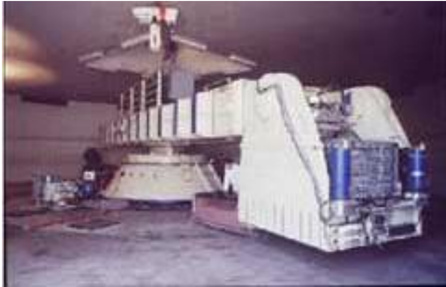
Foto 10. Maquina centrifuga con radio de 9 metros. Modelling Of Earthquake Damage Using Geotechnical Centrifuges, S. P. Gopal Madabhushi
