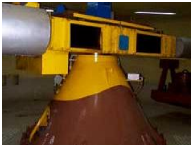
Foto 11. Maquina centrifuga con radio de 4.5 m. Modelling Of Earthquake Damage Using Geotechnical Centrifuges, S. P. Gopal Madabhushi
