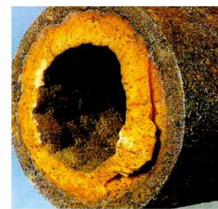
Figura 3. Deposición de parafina. Tomado de: Andrzej, A. et al. (2001). Emergence of flow assurance as a technical discipline specific to deepwater: Technical challenges and integration into subsea systems engineering.
