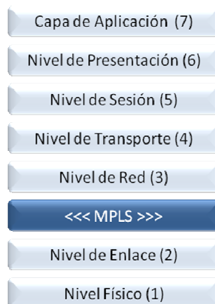
Figura 3. Modelo OSI 1 (fuente Multiprotocol Label Switching Architecture. Network Working Group)
