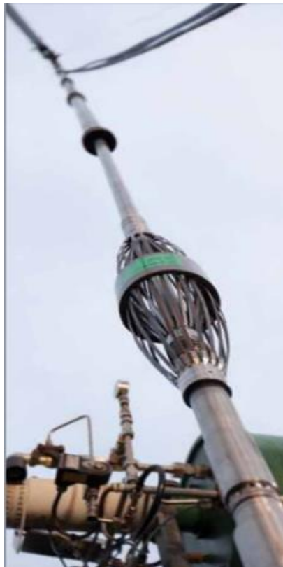
Figura 23. Electromagnetic casing inspection.
