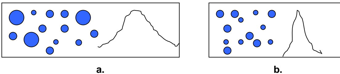
Figure 16. Hydrogels with similar mean pore size but different PSD. a. Broad PSD. b. Narrow PSD.
