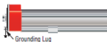
Figure 3. EP Sensor grounding lug location
