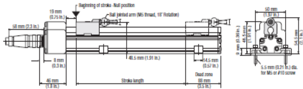
Figure 4. E-Series Model EP sensor dimension reference (Shown with Style V captive-sliding magnet)
