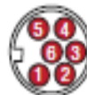
Integral D6 connector (male) as viewed from the end of the sensor
