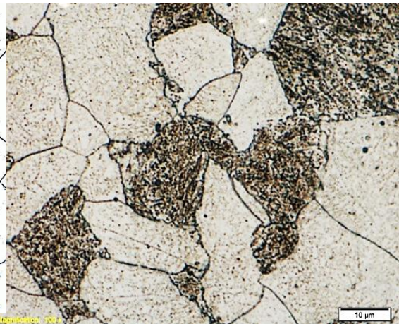
Figura 12: Ferrita, Perlita y bainita. Nital 2%. 2000x
