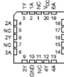
SN54ALS04B, SN54AS04 ... FK PACKAGE (TOP VIEW)
