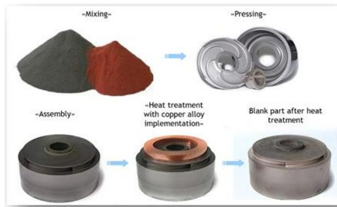
Fuente. Powder Metallurgy Stages Manufacturing Technology Novomet.
