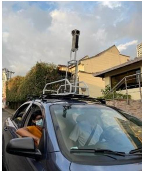
**Figura 46.** Prueba de Panoramas a diferentes Alturas
