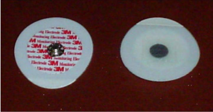
Figura 11. Electrodo Ag- AgCl
