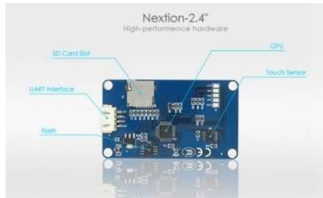
Figura 17. Pantalla NX3224T024_011R - 2.4" TFT LCD TOUCH. Nota. Tomado de: NEXTION NX3224T024 - GENERIC 2.4"TFT INTELLIGENT LCD TOUCH DISPLAY. Disponible en: https://www.itead.cc/nextion-nx3224t024.html .
