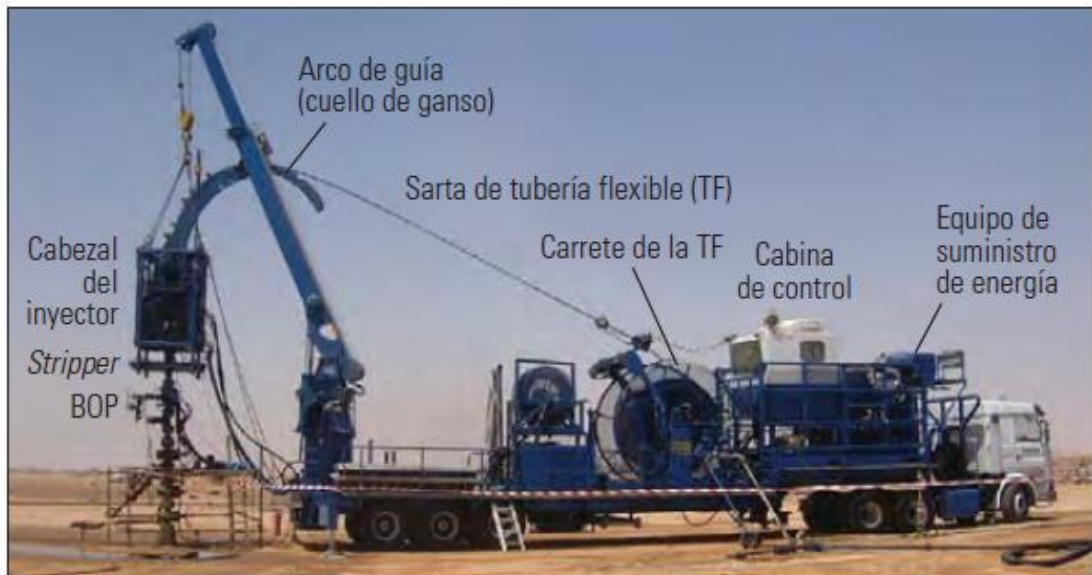
Figura 2 Unidad de coiled tubing.
