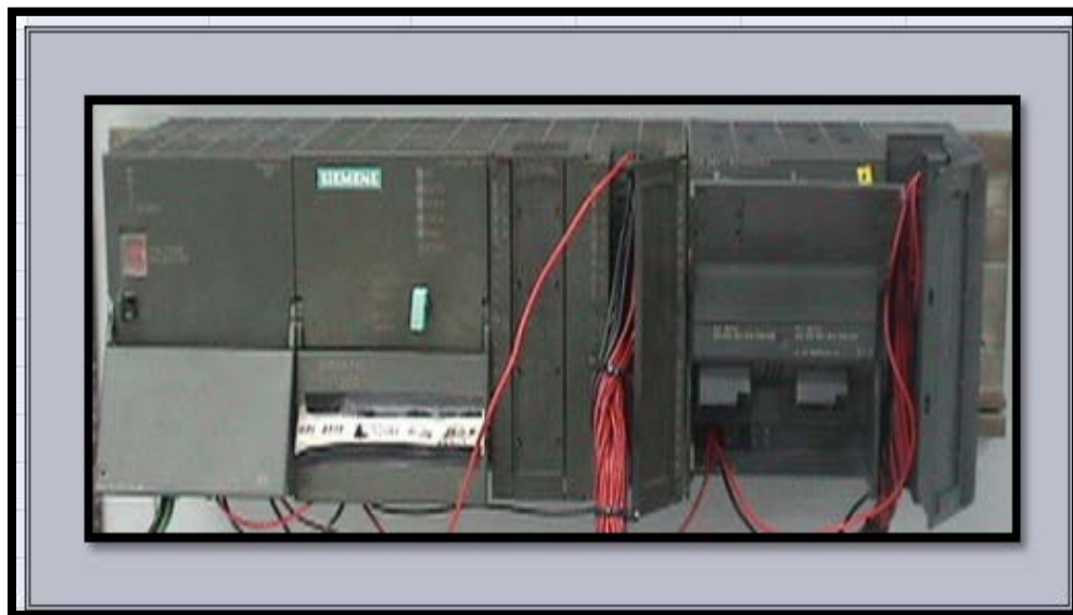
Figura 10. Automata programable 314 IFM
