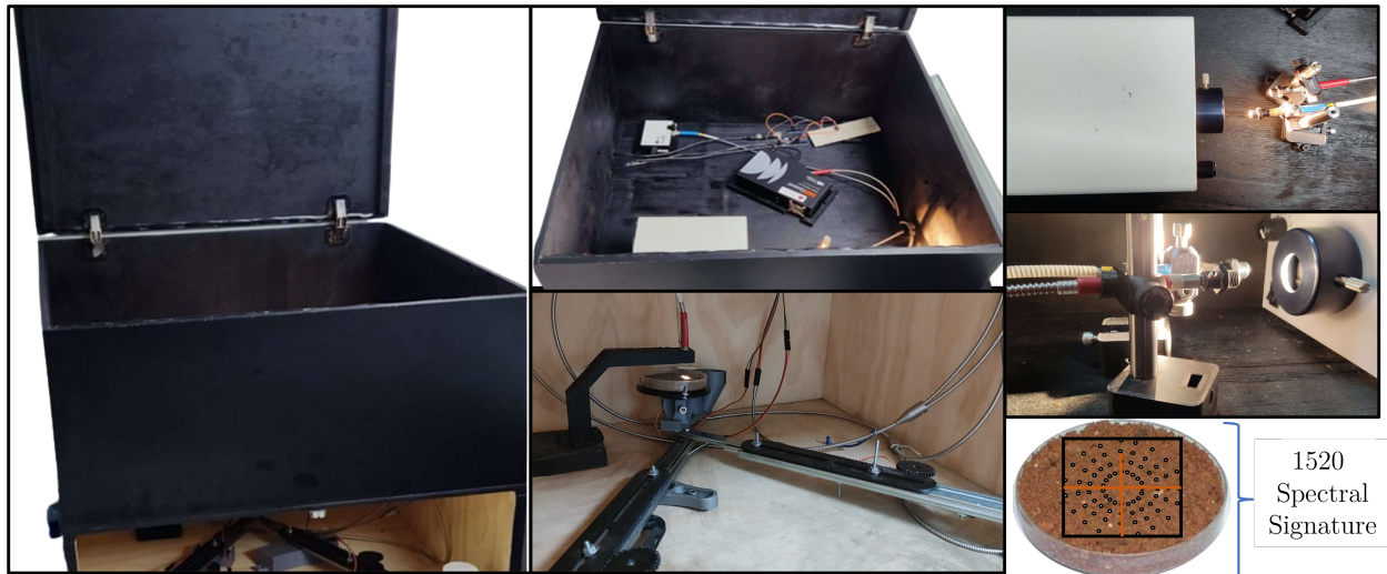
Figure 18. Prototype 1: Construction and implementation of an automated spectral acquisition system.
