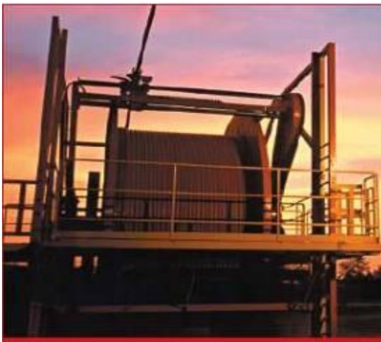
Figura 17. Carrete del coiled tubing.
