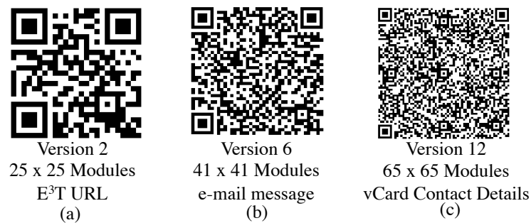
Figure 2.2: QR code version. (a) QR code version 2 of 25 \times 25 modules, encoding E3T URL address. (b) QR code version 6 of 41 \times 41 modules, encoding an e-mail message. (c) QR code version 12 of 65 \times 65 modules, encoding a vCard contact information
