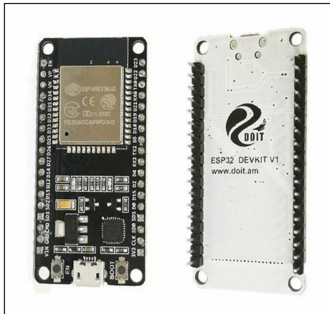
Basado en Figura: Development board created by DOIT, Esp32 DevKit v1
