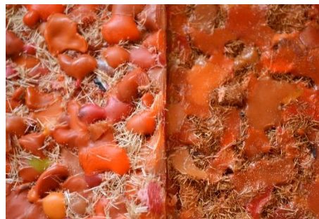
Figura 25: PEAD + 10% Figue a 220°C
