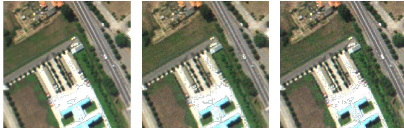
Figure 15: Spatial fusion results. (Left) Reference image. (Middle) Sparse Fusion result. (Right) Proposed fusion approach (Compression ratio of 0.5).
